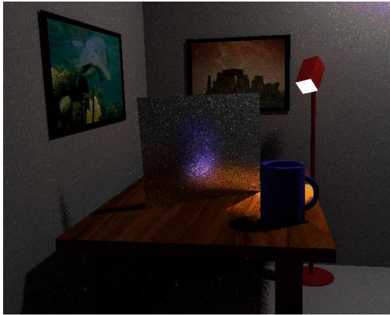
Plate A.4: An image using Monte-Carlo path tracing to compute the global illumination. The mug on the table is reflected in a brushed metal plate. The shader describing the material of the plate uses a highly specular Phong reflection model, which is sampled appropriately by the Monte-Carlo technique. (Color version of Figure 6.8 on Page 130).
