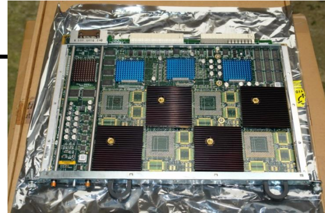
SGI Infinite Reality Geometry Engine (approx. 51x48 cm)
