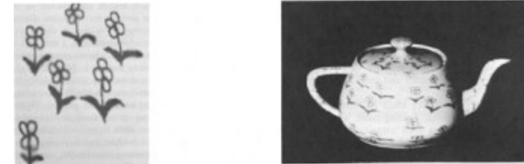
Fig. 4. Photographic texture patterns: left-hand side shows texture patterns; right-hand side shows textured object
