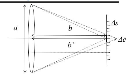
Sharpness criterion based on pixel size and CoC
