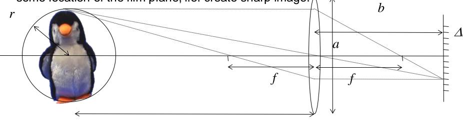
Lens formula defines reciprocal focal length (focus distance from lens of parallel light)
