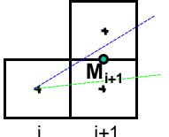
IF  $(d_{i+1} \le 0)$  // Increment in x only  $d_{i+2} = d_{i+1} + a = d_{i+1} + dy$  // Incremental calculation ELSE // Increment in x and y  $d_{i+2} = d_{i+1} + a + b = d_{i+1} + dy - dx$  y = y + 1ENDIF x = x + 1
