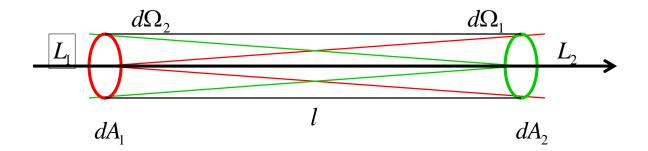
Flux leaving surface 1 must be equal to flux arriving on surface 2  $L_1 d\Omega_1 dA_1 = L_2 d\Omega_2 dA_2$
