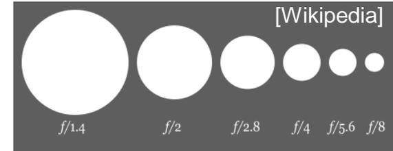
Doubling the f-number decreases the aperture area by a factor of four (i.e. need to quadruple exposure time to preserve same brightness)
