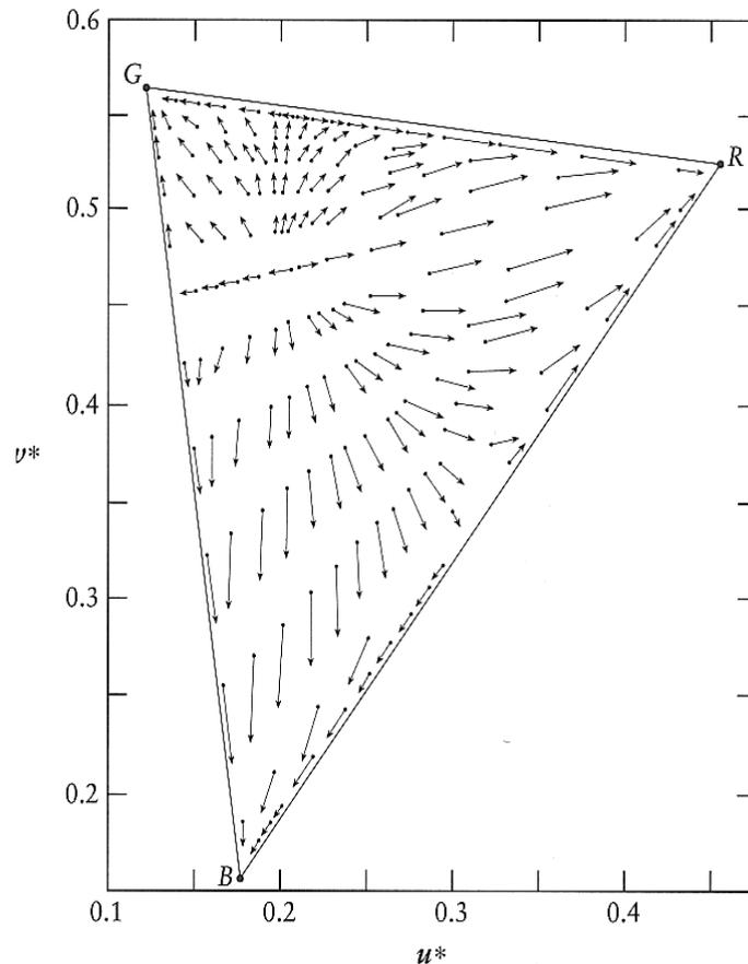
Shifts in reproduced chromaticities resulting from uncompensated gamma of 1.273 (such a gamma is desirable to compensate the contrast lowering in the dim surround).
