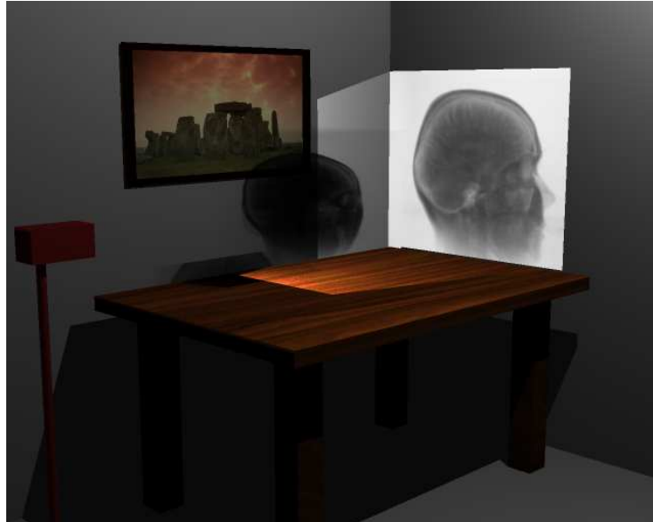
Plate A.8: An image showing the integrated rendering of surface and volume data in the Vision architecture. This image was rendered with direct illumination and a ray tracing renderer. The volume object above the desk is projected onto the wall and the desk as well as viewed directly. (Color version of Figure 6.25 on Page 162).
