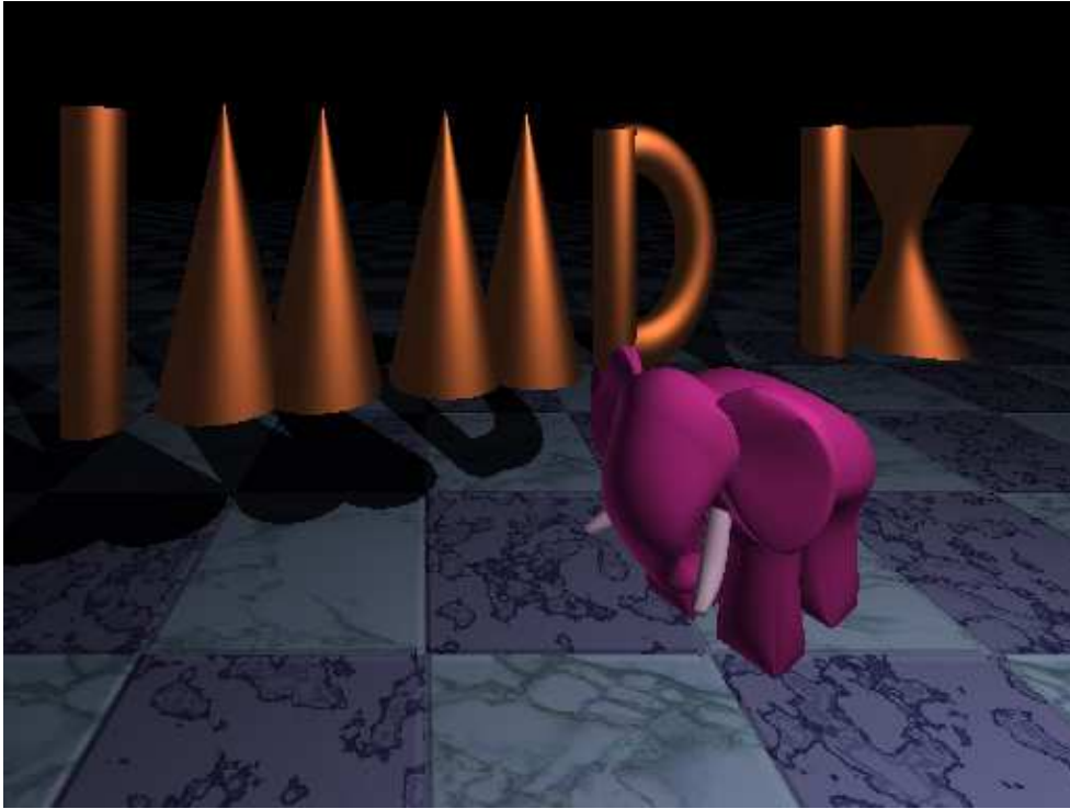
Plate A.12: Three recursive shaders applied to the floor. The checker board shader calls two different marble shaders and performs bump mapping at the edges of the tiles. (Color version of Figure 8.2 on Page 205).
